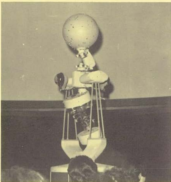
Constellations were projected onto the dome of the planetarium through small holes in this piece of equipment.
